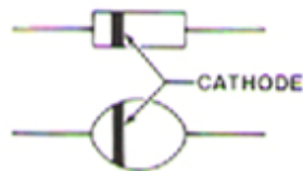
CATHODE MARKED WITH A BAND
